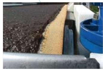
*Separated particles transported to top of belt and drained to high matter content*
