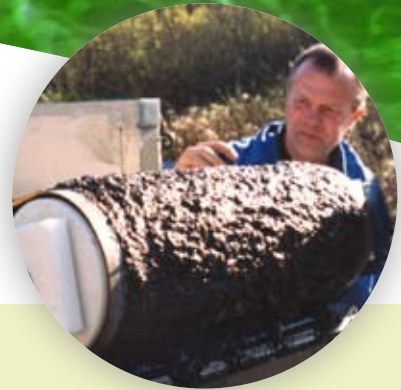
Concentrated sludge after filtration with the Hydrotech Beltfilter
