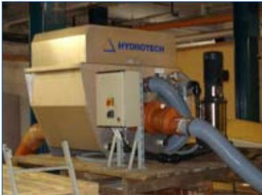
*Testing Drumfilter at an eel farm*
