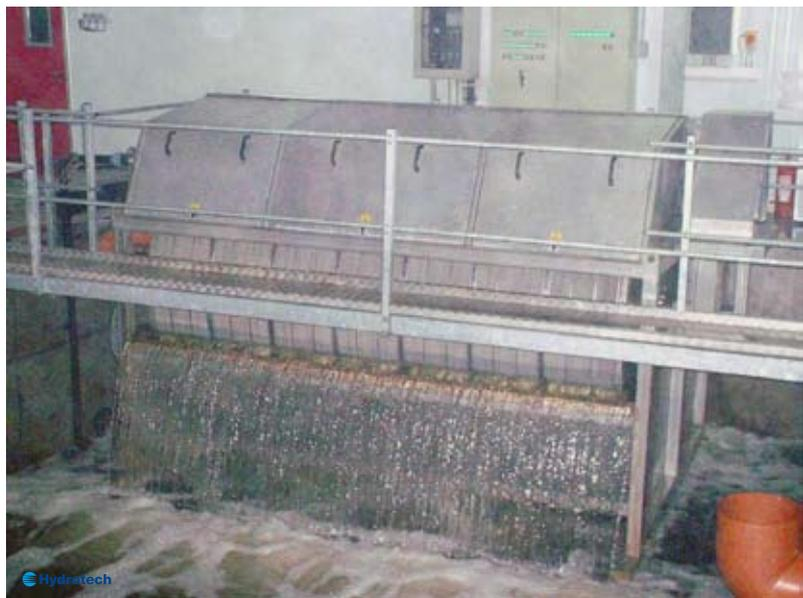
*HDF2007-1A, installed on top of a moving bed biofilter*
